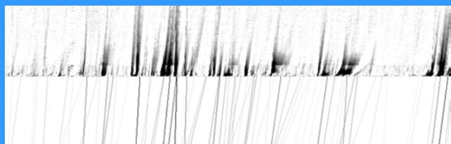
CMEs can be seen in [height, time] plots (top) as inclined ridges with the inclination angle corresponding to the propagation speed. Time runs horizontally over May, 1998, the vertically height covers the combined C2/C3 FOV. The ridges are detected with the Hough transform (bottom).
