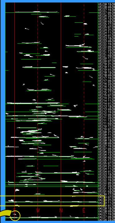
In this combined map we show the 95 events found by the software (white) as compared to the 71 CMEs reported in the catalogs (green). Time is running vertically over May, 1998. The horizontal dimension is the poloidal angle around the sun, the left side corresponding to the C3 occulter.
