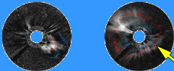
By combining the ridges in [height,time] plots from all directions, one can reconstruct the CME front as it propagates outwards. The red lines in the above images track the front of a fast halo CME (left) and a slow, regular CME (right). The blue and yellow lines correspond to the position of the front at earlier and later times, giving an indication of the time evolution.
