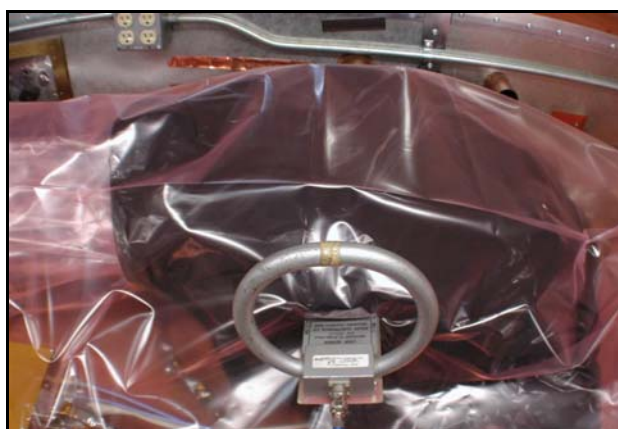
Figure 11-8. RE01 Setup for MAG Sensor Testing
