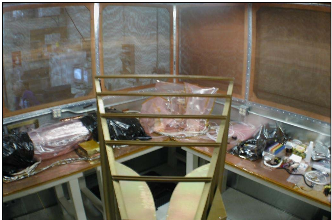
Figure 12-7. RE02 SAS-570 Double Ridged Horn Antenna Position #1 (200 MHz – 1 GHz)
