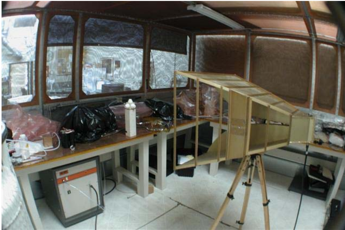
Figure 13-4. Configuration for RS03 Testing on the Stereo Impact (200 – 1000 MHz) - Vertical Polarization
