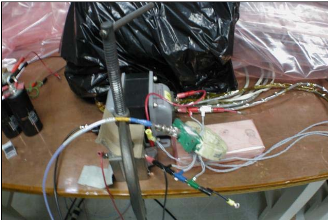
Figure 8-3. Close-up of Injected Signal Monitoring Instrumentation During CS01 Testing (30 Hz – 51 kHz)
