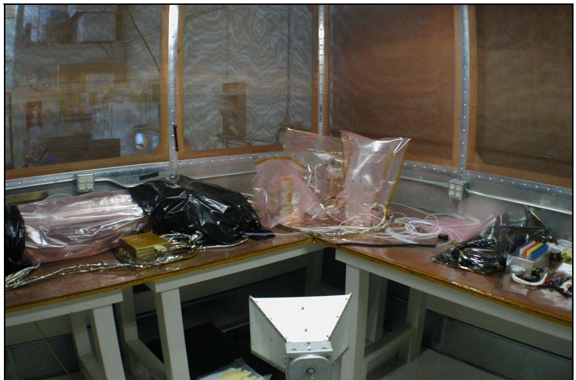
Figure 12-9. RE02 EMCO 3115 Double Ridged Horn Antenna Position #1 (1 GHz – 10 GHz)
