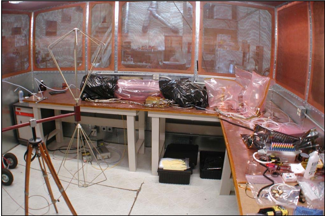
Figure 12-4. RE02 Vertical Biconical Antenna Position #1 (30 MHz – 200 MHz)
