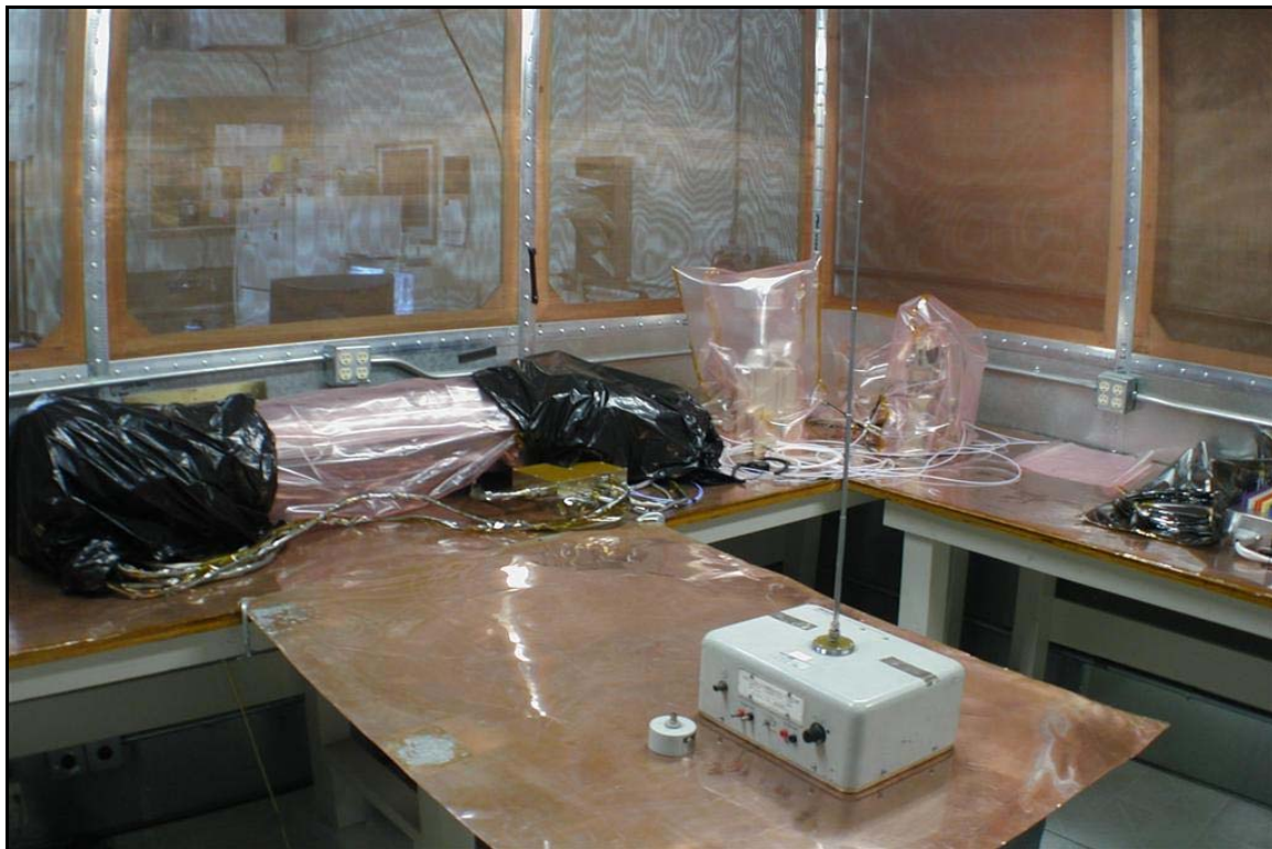
Figure 12-2. Configuration for Stereo Impact RE02 Testing with the Monopole Antenna (2 kHz – 30 MHz)
