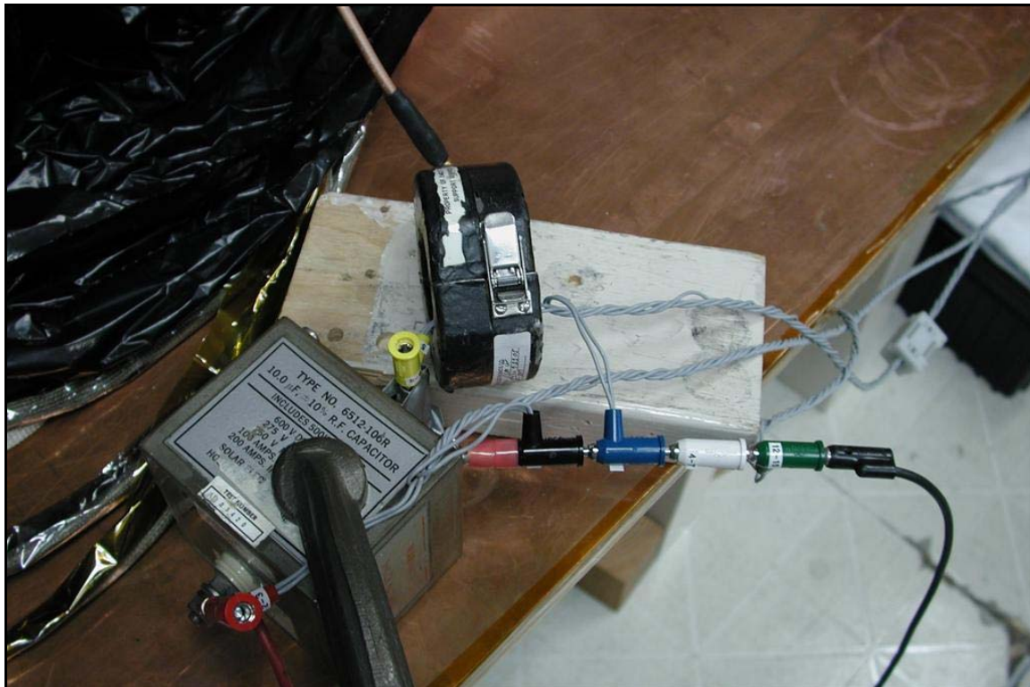
Figure 5-3. Close-up of STEREO IMPACT Input Power Lead (Differential Mode)
