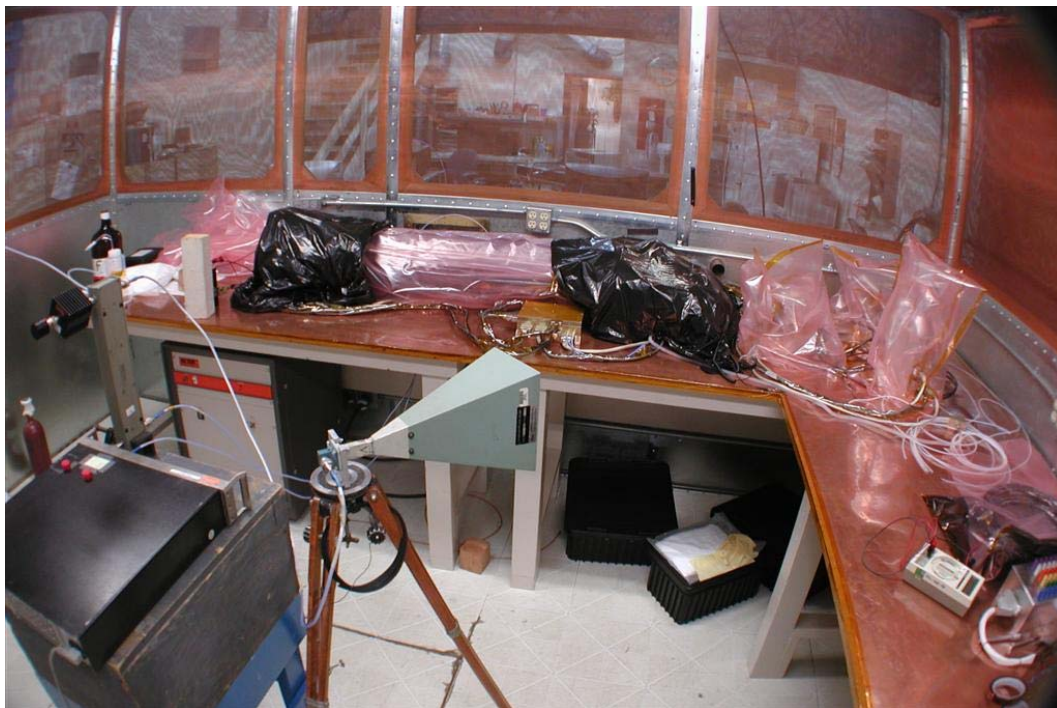
Figure 13-9. Configuration for RS03 Testing on the Stereo Impact (8 – 12 GHz) - Horizontal Polarization– Antenna Position #1
