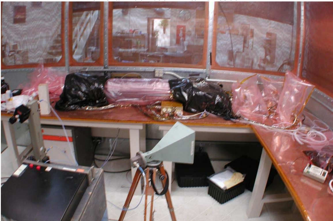
Figure 13-7. Configuration for RS03 Testing on the Stereo Impact (4 –6 GHz) - Horizontal Polarization – Antenna Position #1
