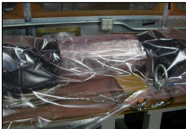
Figure 11-6. RE01 Setup for IDPU Testing
