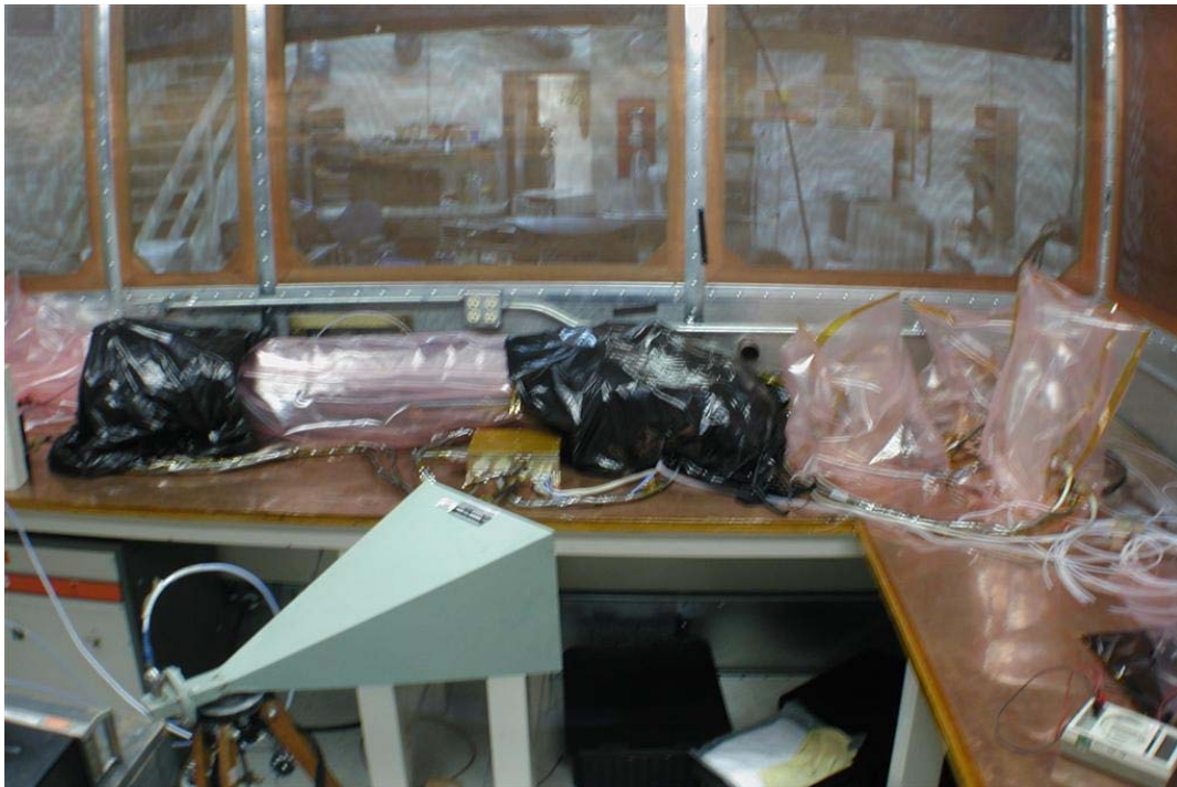
Figure 13-8. Configuration for RS03 Testing on the Stereo Impact (6 – 8 GHz) - Vertical Polarization – Antenna Position #1
