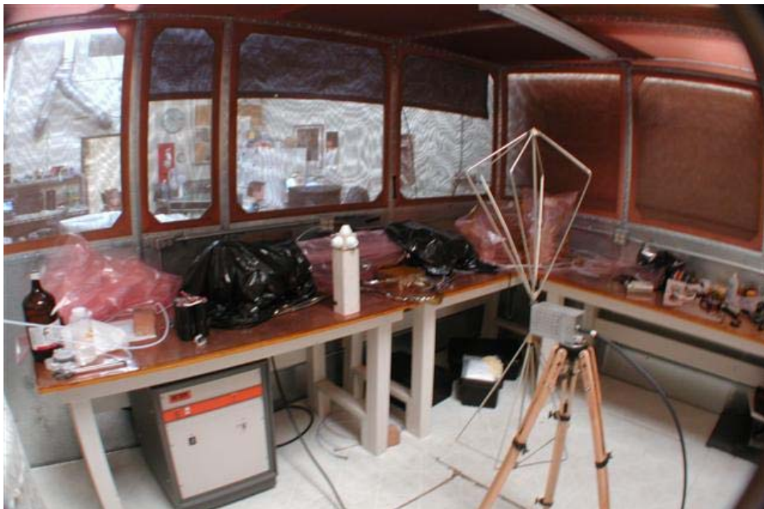
Figure 13-3. Configuration for RS03 Testing on the Stereo Impact (30 – 200 MHz) - Vertical Polarization
