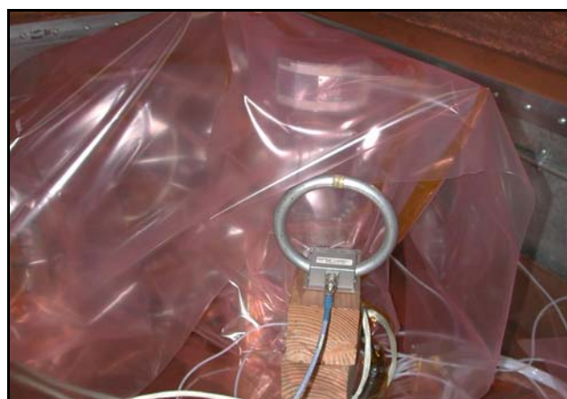
Figure 11-10. RE01 Setup for SEP Central/HET/LET (Antenna is close to the HET Unit)
