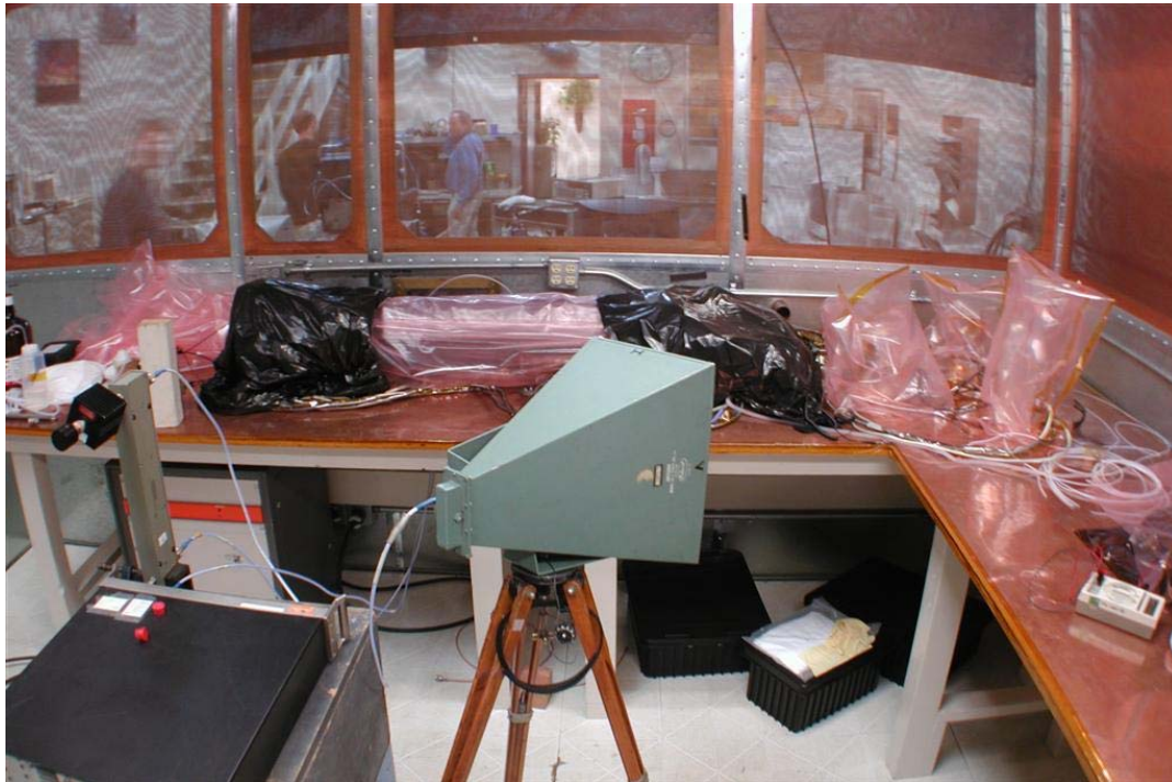
Figure 13-6. Configuration for RS03 Testing on the Stereo Impact (2 –4 GHz) - Horizontal Polarization – Antenna Position #1
