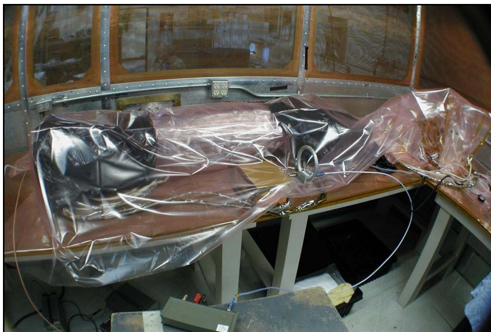
Figure 11-4. Loop Antenna Configuration for RE01 Testing(30 Hz – 49 kHz)
