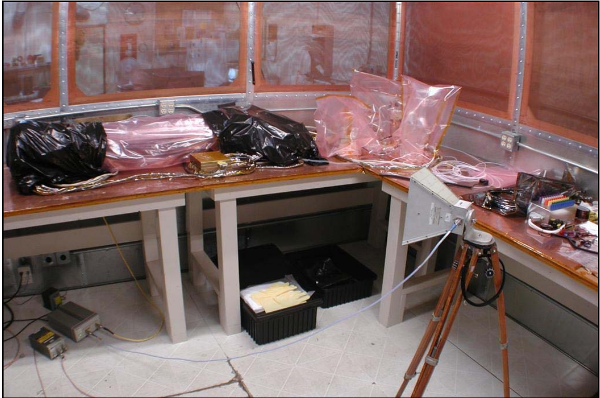
Figure 12-8. RE02 EMCO 3115 Double Ridged Horn Antenna Position #2 (1 GHz – 10 GHz)
