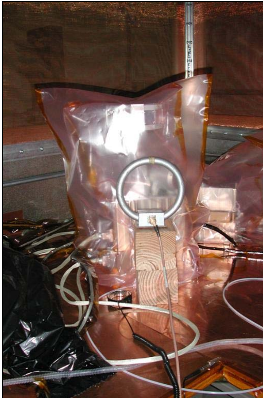
Figure 11-5. Close-up of the RE01 Magnetic Field Loop Testing on the SEP Central/HET/LET Units (30 Hz – 49 kHz) (Antenna is close to the HET Unit)
