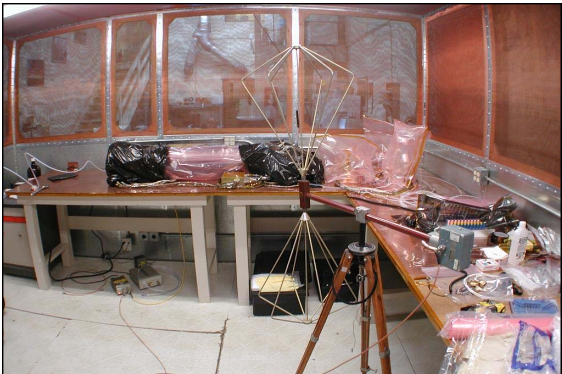
Figure 12-5. RE02 Vertical Biconical Antenna Position #2 (30 MHz – 200 MHz)
