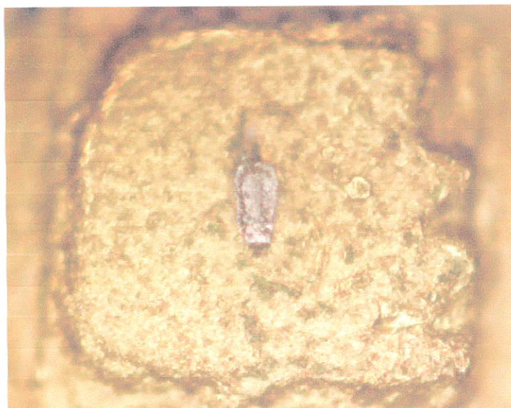
Figure 10. Optical and SEM images of the wire bond “foot” present on diode D8.
