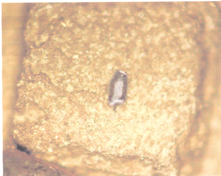
Figure 9. For comparison, optical and SEM images of the wire bond “foot” present on diode D7 are shown above.
