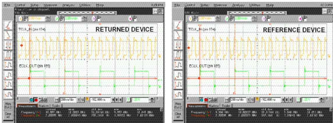
Figure 9: Scope plot of the output signal eclk_out (pin 189) of the returned device (LEFT) is identical to that of the reference device (RIGHT) when the charge pump is turned on by the test program
