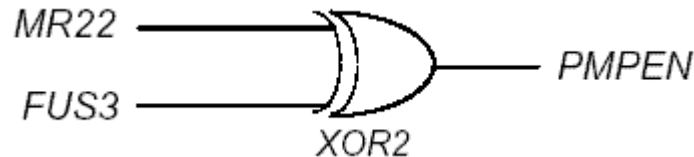
Figure 10: Circuit generating the PMPEN (pump enable signal)
