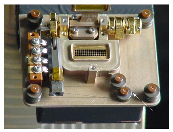
The door was again actuated with the cover off and a much smoother and somewhat faster motion was observed. The pulley was observed to rotate normally. A 100-cycle test was performed while monitoring the actuation time and the door motion. The door continued to operate smoothly and the actuation time showed no trends.
