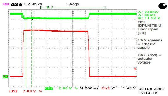
STE-U FM1 door open attempt (fails). Green trace is the supply that powers the door actuator; the voltage sag is within spec and as measured previously. The red trace is the voltage on the actuator (after a 15 ohm series resistor), and is also normal (the actuator resistance is ~55 ohms). The door power continues till timeout after 1 second without completing the door motion (normally when the door reaches the open position a sense switch closure causes the actuator power to be discontinued).
