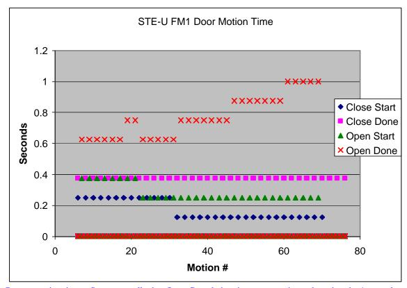
Door actuation times. Starts normally, but Open Completion time starts to rise and reaches the 1 second timeout after  $\sim$ 70 motions (1 open/close cycle is two motions). There is also a small downwards trend in the time it takes to start moving in both directions that may be significant. Note that the time measurement resolution is 1/8 second.
