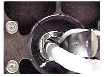
These pictures show that the modifications done to the pinpuller mounting ring are sufficient to remove the galling between it and the tip piece.
