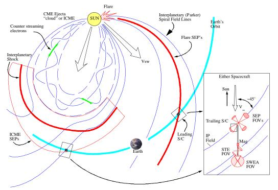
Fig. B.1 The measurement and science domain of the STEREO IMPACT investigation. IMPACT detects solar wind plasma electrons, including the heat flux electrons that can be used to trace magnetic field connections to the Sun, the local magnetic fields, and energetic ions and electrons generated at the Sun in flares and at CME-generated interplanetary shocks.
