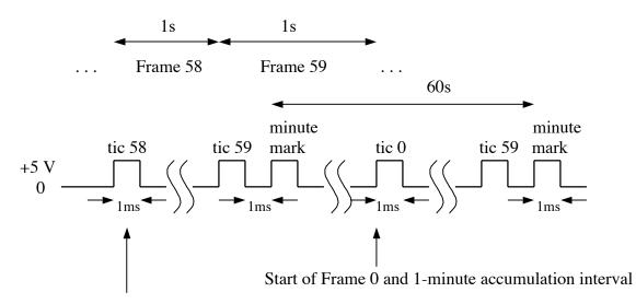
FRAME SYNC: active high, 1s period, nominally 1ms long; double-pulsed every 60s to provide the 1-minute mark
