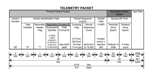
Figure 11. CCSDS Telemetry Packet Data Structure Diagram
