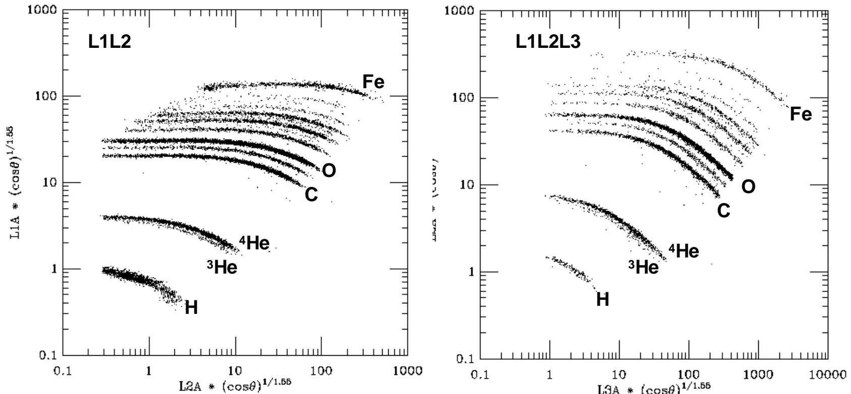
Scatter plot of simulated pulse-heights from the L1 vs. L2 and the L2 vs. L3 detectors on LET illustrating particle tracks from H to Fe. The resolution and calibration of the LET system must be sufficient to resolve the tracks of these and other species and measure their kinetic energy.
