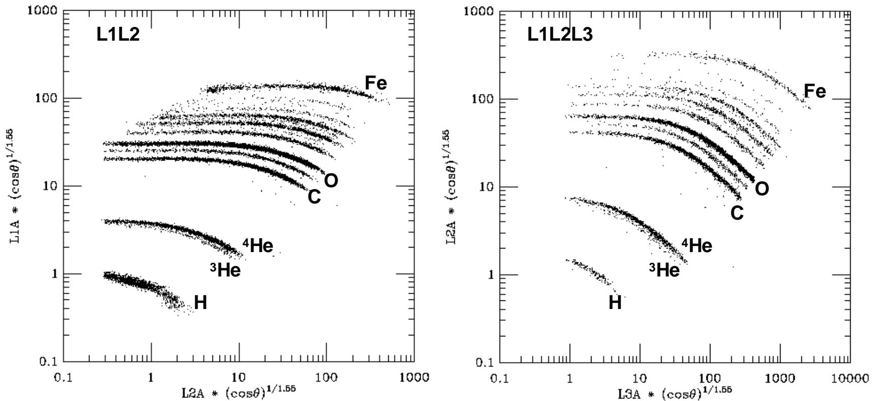
These simulations include the effects of Landau fluctuations as well as variations in the angle of incidence and detector-thickness uniformity ( $S_T = 0.5$  microns in L1, L2). All key species are resolved. Note that incidence-angle and detector-thickness corrections will be made onboard.
